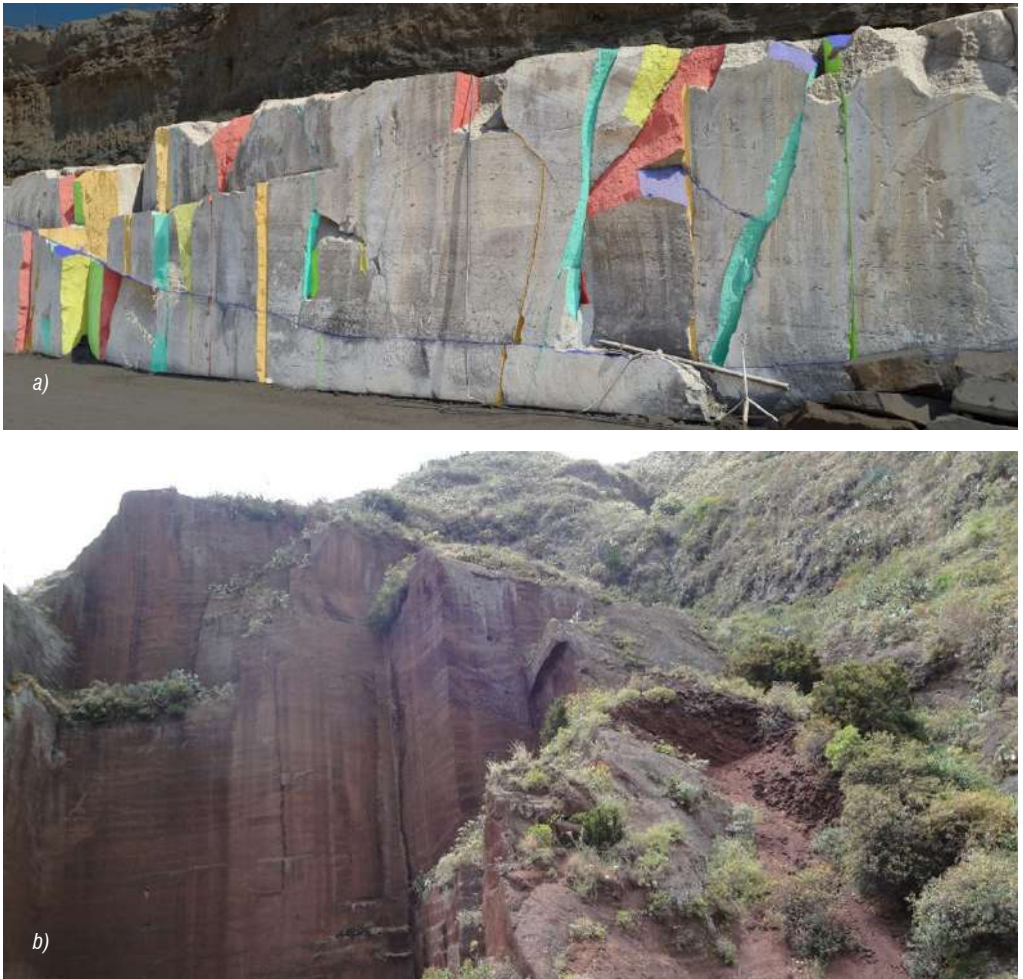
Fig 1. Example of fracture pattern in an ignimbrite quarry (a); historic quarry in tuff outcrops (b).
