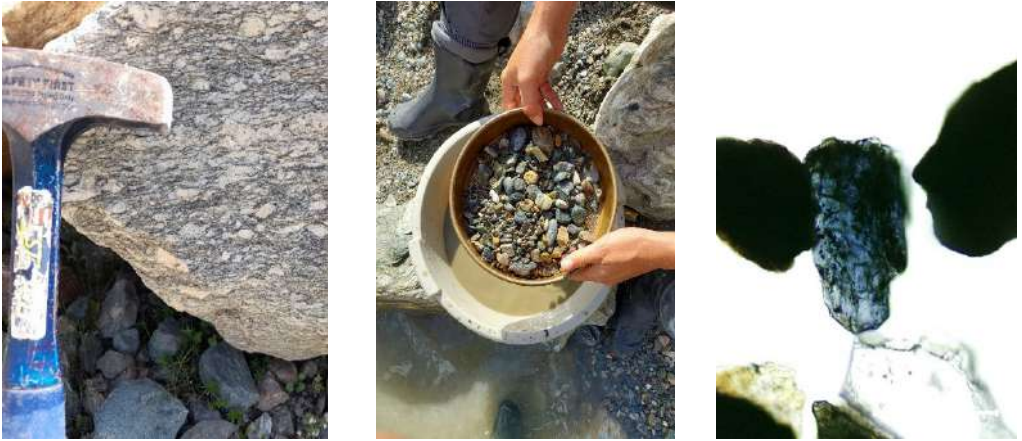
Fig 1. Samples recovered within the project, a) an augen gneiss, b) stream sediments; c) optical image of a heavy mineral fraction showing glaucofane in PPL (center).
